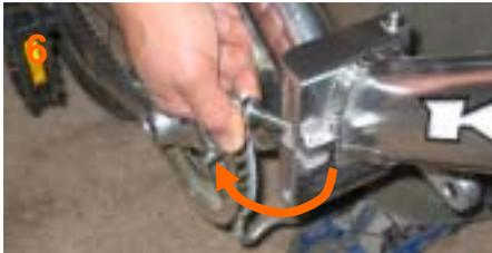
6. Open the quick-release on the main body. Then turn the quick-release lever toward the back end of the bike.
