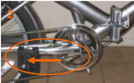
2. Rotate the crank so that the folded pedal is pointing toward the rear wheel.
