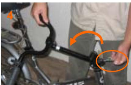
4. Turn the quick-release lever onto a horizontal position (circled) to disengage the safety latch, then fold down the head-stem. If you have a Mocha, be careful that the cables do not snag on the folding mechanism.
