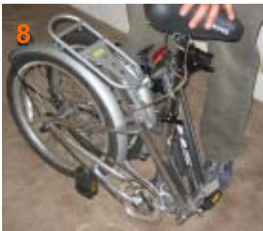
8. Fold the bike in half. If you have Mocha, be careful that the cables do not snag on the folding mechanism.
